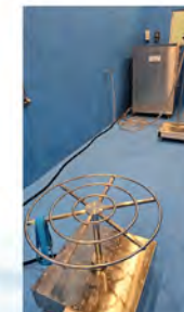
IPX5 & IPX6 Waterproof Jet Test Device
