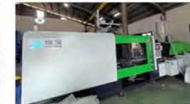
360 Ton Plastic Injection Moulding Machine
