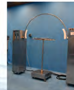
IPX3 & IPX4 Swing Pipe Water Spray Test
