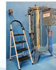
IPX7 & IPX8 Immersion tank Waterproof Test Device
