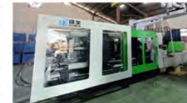
800 Ton Plastic Injection Moulding Machine
